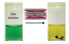
Selective and efficient adsorption is achieved with a porous nanostructured liquid crystalline polymer network. The confined pore dimensions allow charge and size selective adsorption and the smectic porous nature results in fast accessibility of all adsorption sites.
