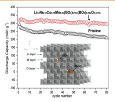
As-prepared  $Li[Li_{0.2}Ni_{0.13}Co_{0.13}Mn_{0.54}]$  $(BO_4)_{0.015}(BO_3)_{0.005}O_{1.925}$  shows a decreased M-O covalency and a lowered O 2p band top compared with pristine  $Li[Li_{0.2}Ni_{0.13}Co_{0.13}Mn_{0.54}]O_2$ . As a result, the modified cathode exhibits a superior reversible capacity of 300 mA h g<sup>-1</sup> after 80 cycles, excellent cycling stability with a capacity retention of 89% within 300 cycles, higher thermal stability, and enhanced redox couple potentials.
