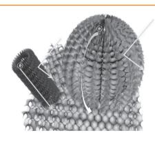
Hierarchical double-shell nanostructures consisting of TiO2 nanosheets on SnO2 hollow spheres are prepared to provide large surface area, excellent electron transport, and improved light scattering. The resulting solid-state dye-sensitized solar cells show enhanced efficiency up to 8.2% at 100 mW cm<sup>-2</sup>, one of the highest values observed for N719 dye.
