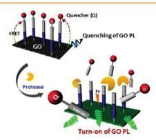
A graphene oxide (GO) fluorescencebased protease sensor consisting of a luminescent GO donor conjugated with a peptide-quencher complex detects cellsecreted proteases. The most effective quencher for GO fluorescence creates a GO-peptide-QXL optical sensor for protease detection. The quenched fluorescence of GO is restored by the proteolytic cleavage of a peptide quencher moiety from the sensor. This "turn-on" optical sensor detects MMP-2 secreted from live cells with high sensitivity.
